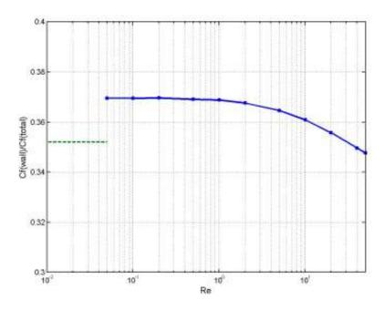
Fig. 1 Variation with the Reynolds number of the relative contribution of the wall shear force. [1] Brenner, H., *Chemical Engineering Science*, pp. 519-539, 1964.
