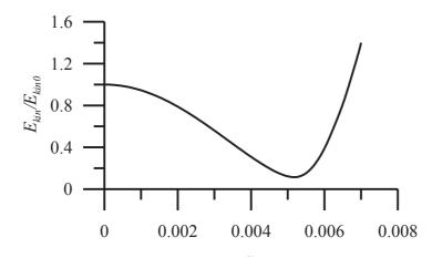
Fig. 1 The dependence of kinetic energy of the fluid motion on the dimensionless amplitude of vibrations for Pr = 0.02, Re = 2059, We = 17000
