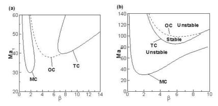
Fig. 1 Marginal curves of the system in Ma-k plane for Different Biot numbers: (a) Bi=30 and (b) Bi=300, at same depth ratio  $h(h_1/h_2)=0.5$ , and streamwise disturbance wavenumber  $\alpha=0$ . The dashed lines correspond to the oscillation mode and the solid lines represent the stationary mode.
