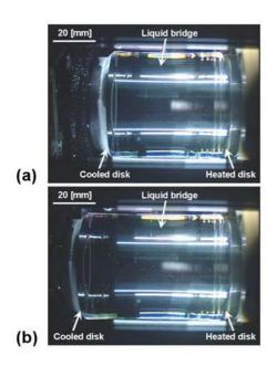
Fig.1. Side view of liquid bridge of 25 mm in radius and of Pr = 206.8 (at 25 °C); (a)  $\Gamma$  = 2.0 and (b)  $\Gamma$  = 2.5.
