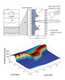
FIG. 1: Top: schematic drawing of the experimental setup: front view (left) and side view (right); Bottom: reconstructed three-dimensional plot from the surface waves with contours shown for  $900\mu m$ ,  $1200\mu m$ .
