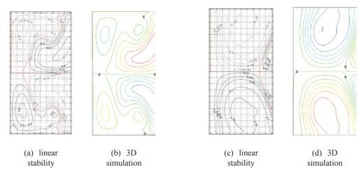
FIG. 2: The stationary m=2 mode for Ha=5 at  $Re_{FZ}=1950$  shown by comparison of three-dimensional simulations to linear stability theory via contours of the azimuthal velocity (left) and the electric potential function (right) over the domain  $1 \le z/b \le -1$  and  $0 \le r \le 1$  in the  $\theta$  plane where each reaches its maximum.
