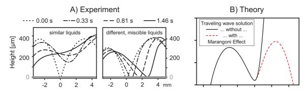
FIG. 1: A) Experimental center-to-center profiles of droplets with instantaneous (left) and delayed (right) coalescence. B) Traveling wave solutions to a thin film equation: classical, semi-infinite solution without surface tension gradient vs. localized (i.e., two droplets) solution with local surface tension gradient (dashed).
