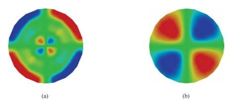
FIG. 1: The stationary m=2 mode for Ha=5 at  $Re_{FZ}=1950$  shown by a) the azimuthal velocity and b) electric potential at z/b=0.5.
