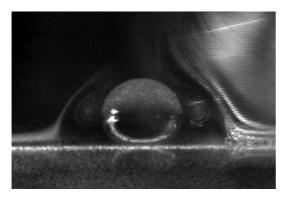
Fig. 1 Image of levitated microliter-volume silicone oil droplet with visualization of surrounding flow field
