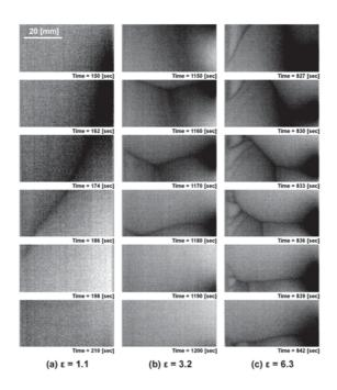
Fig.2. Time series of temperature deviation on the liquid bridge surface of 1/6 region in azimuthal direction evaluated by IR images in the case of  $\Gamma = 2.0$ ; (Ma,  $\varepsilon$ ) = (a)  $(4.2 \times 10^4, 1.1)$ , (b)  $(8.5 \times 10^4, 3.2)$  and (c)  $(1.5 \times 10^5, 6.3)$ .
