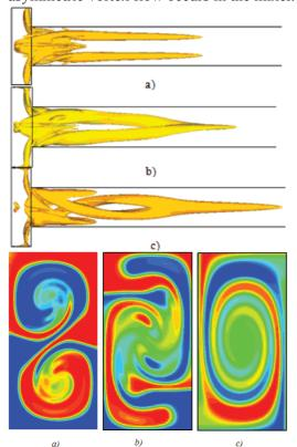
Flow vortex structure and contours of mass fraction of dye in the outlet of microchannel at various value of the slip length b. Re = 186. a) b = 0; b) b = 10  $\mu$ m; c) b = 30  $\mu$ m.
