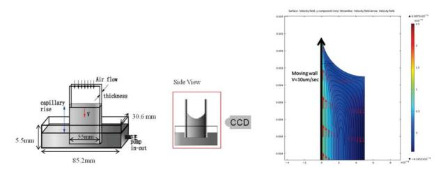
FIG. 1: Left: experimental set-up - Right: Simulation results: Flow field for a polymer solution drying on a moving substrate.
