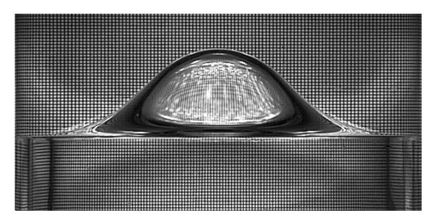
Fig. 1 Experimental excitation of (0,1) cylindrical mode in an immiscible liquid system
