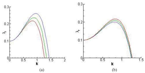
Fig. 1 Effective growth rate  $\lambda_r$  versus the disturbance wave number k. (a) for different effective pressures:  $A_2=0.04$  (red line),  $A_2=0.02$  (green line), and  $A_2=0$  (blue line); (b) for different energy flux:  $\overline{N}=0$  (red line),  $\overline{N}=0.15$  (green line), and  $\overline{N}=0.3$  (blue line). Both the two figures are plotted under the same evaporation number  $\overline{E}=0.1$ , and Reynolds number  $Re=5\sqrt{2}/2$ .
