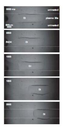
Fig. 1: Droplet actuation on a hydrophilic stripe.
