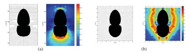
Fig.1. Flow field (left subplots) and flow intensity (right subplots) around a coalescing doublet system during its quasi-static motion. (a) The trailing drop reached the leading one, but coalescence has not yet begun; (b) Immediately after coalescence starts. Frames are taken 0.2 s apart.
