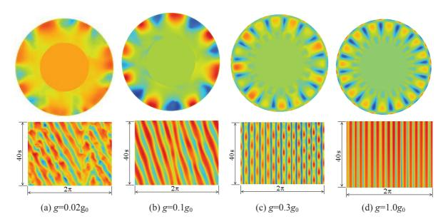
Fig. 1 Flow pattern transition process at  $\Delta T$ =10K. Upper plot: snapshots of surface temperature fluctuation; Down plot: space-time diagram of surface temperature distribution at a given radius
