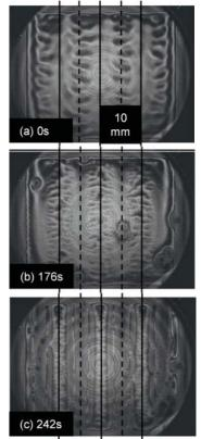
Fig. 1. Phase-shifting shlieren images of an evaporating film of a fluorinert liquid HFE 7500 on a heated structured wall. Solid line: structure trough; dashed line: structure crest.
