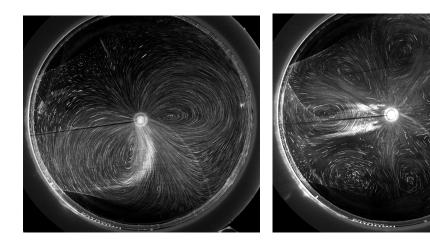
FIG. 1: The surface flow structure under  $Ma=2\cdot 10^6$  and surfactant surface density  $\Gamma/\Gamma_e$ =0.35 (left picture) and 0.3 (right picture).  $\Gamma_e$  - surface density of monolayer.
