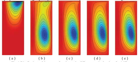
Fig. 1 Distributions of the stream function at the different gravity levels at  $B_0$ =1.0T. (a) G=0,  $\psi_{\text{max}}$ =0.400×10<sup>-7</sup> m<sup>3</sup>/s. (b) G=0.1g,  $\psi_{\text{max}}$ =0.723×10<sup>-7</sup> m<sup>3</sup>/s. (c) G=0.5g,  $\psi_{\text{max}}$ =1.51×10<sup>-7</sup> m<sup>3</sup>/s. (d) G=0.8g,  $\psi_{\text{max}}$ =1.78×10<sup>-7</sup> m<sup>3</sup>/s. (e) G=g,  $\psi_{\text{max}}$ =1.91×10<sup>-7</sup> m<sup>3</sup>/s.
