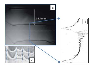
FIG. 1: Typical two-dimensional waves in water falling films, 140mm downstream of the inlet (dashed line in a)): a) averaged-image of 30 waves; b) CCI film thickness measurement; c) with high heating -dashed lines indicate hot-streaks
